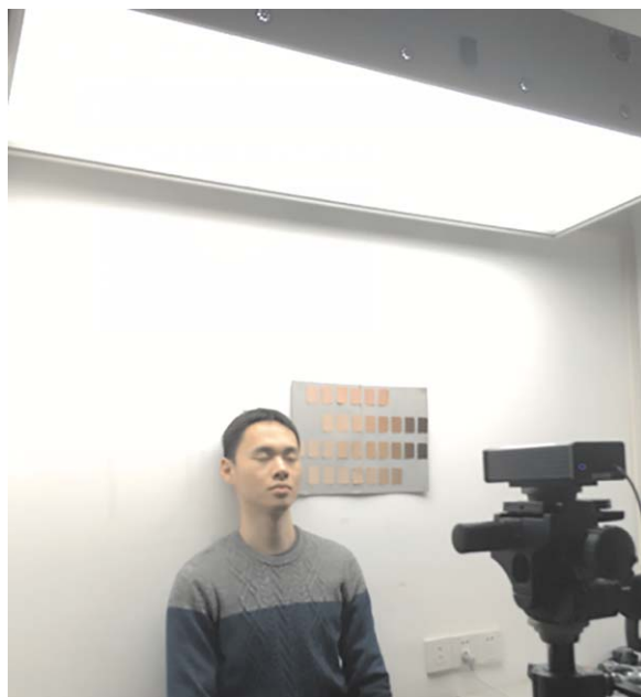
FIGURE 2 Subject in measurement position under a florescent illuminant D65 simulator ceiling light
